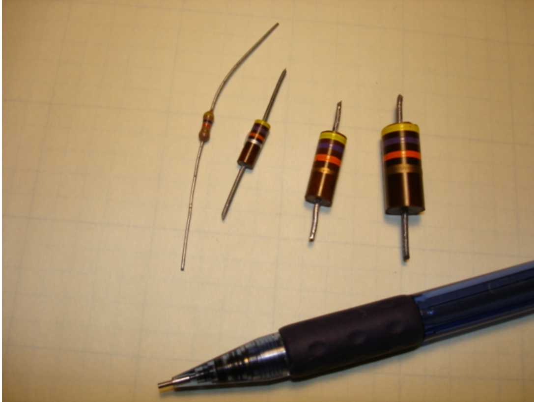
Figure 5. These 47-kohm resistors can dissipate (left to right) 1/4 W, 1/2 W, 1 W, or 2 W. The colored bands indicate the resistance value. Note the size of the pencil for size comparison.
